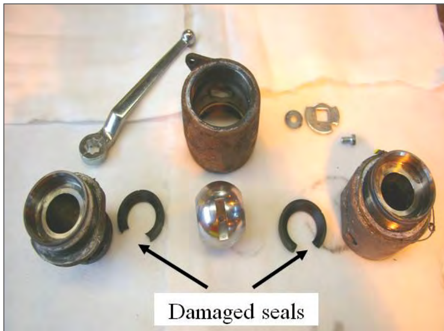
Figure 1 - Damaged Ball valve dismantled showing damage to seals
